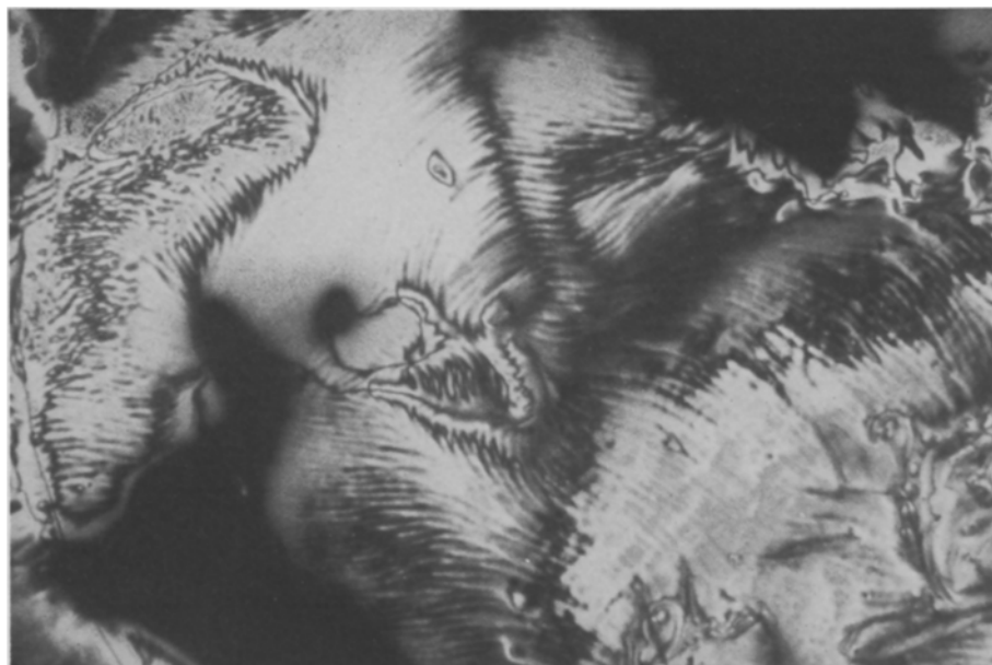
Figure 5 - Photomicrograph of re-entrant nematic phase from polymer PO 6 (crossed polarizers).
